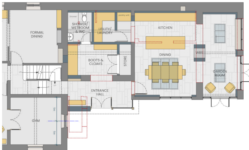
Proposed Ground Floor plan extract with proposed Entrance Hall/Porch providing access to converted spaces
