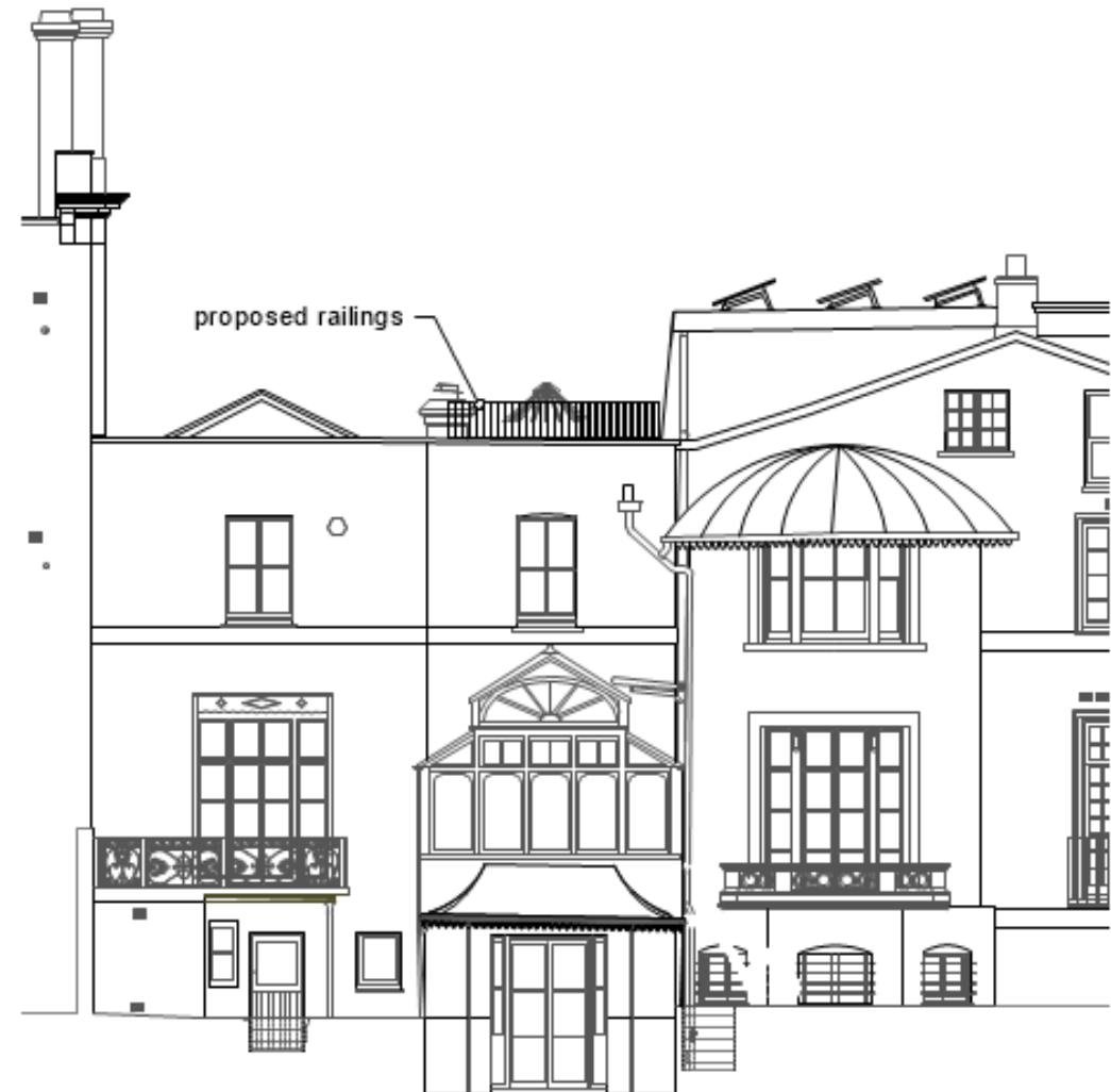
Rear / South East Elevation illustrating the impact of the safety balustrade
