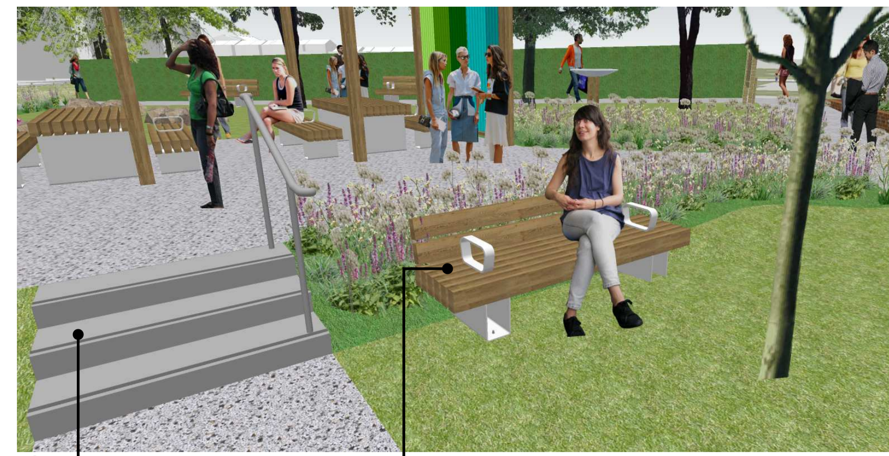
1 STEP UNITS. SUPPLIER: MARSHALLS. PRODUCT CONSERVATION X STEP UNITS. DIMENSIONS: W:1500MM X D:400MM X H:150MM. COLOUR: SILVER W/CONTRAST STRIP. INSTALLED TO SUPPLIERS RECOMMENDATION.
