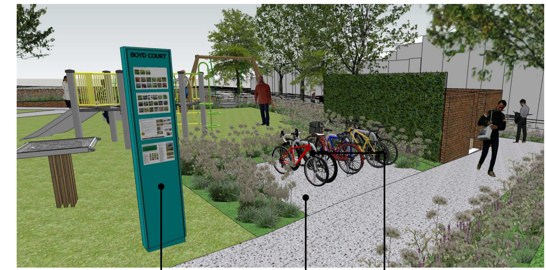
2 SI - SIGN - INFORMATION. SUPPLIER: IS GROUP. PRODUCT: WAY2GO TOTEM CONFIG 3 OR 4. DIMENSIONS: H:2200MM X W:450 X D:140MM. AREA B - TOUGHENED GLASS OVER MAP. AREA D - POWDERCOATED WITH BLUE/TURQUOISE/GREEN. TO INCLUDE: • EACH BOARD WILL HAVE INFORMATION ON THAT PARTICULAR AREA. • OPEN TIME RESTRICTIONS IF ANY. • RULES FOR USING EACH SPACE. • CONTACT NUMBER TO REPORT ISSUES.
