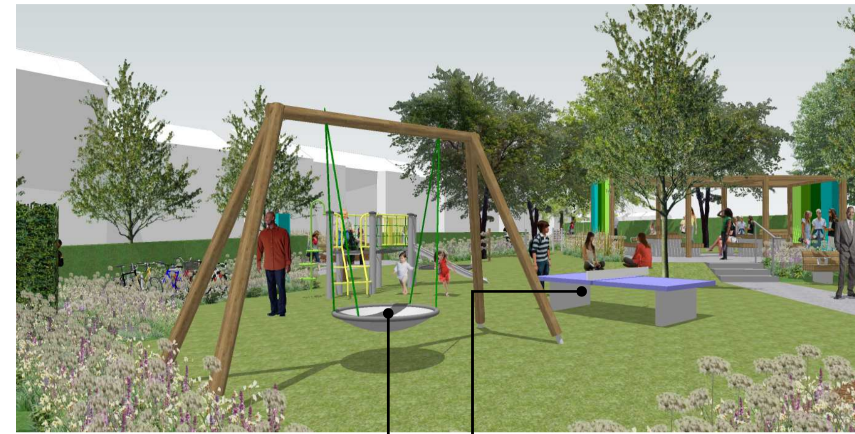
3 BASKET SWING. SUPPLIER: TIMBERPLAY. PRODUCT: 'CRADLE NEST' (6.14520) OR EQUAL APPROVED. TIMBER AND GALVANISED STEEL CONSTRUCTION. INSTALLED TO SUPPLIERS RECOMMENDATION.
