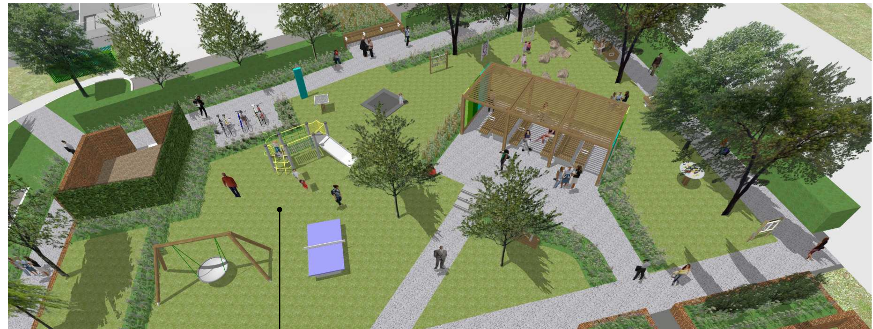
5 SYNTHETIC GRASS. SUPPLIER: EASIGRASS, NAMGRASS OR EQUAL APPROVED. PRODUCT: HOLLAND PARK, ELISE OR EQUAL APPROVED. INSTALLED TO SUPPLIERS RECOMMENDATION WITH SHOCKPAD TO REQUIRED DEPTH TO ALLOW FOR PLAY EQUIPMENT FALL HEIGHTS. SUB-BASE TO ENGINEERS SPECIFICATION.
