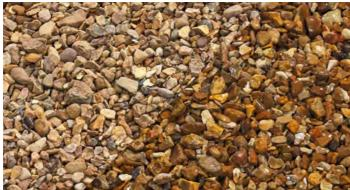
B GRAVEL. SUPPLIER: CED. PRODUCT: QUARTZ GRAVEL. DIMENSIONS: 20MM. LAID INTO A CLEAR PLASTIC 30MM ECCOGRAVEL CELL SYSTEM (SUPPLIER CED) TO REDUCE MOVEMENT WITH AN ADDITIONAL 20MM COVER TO HIDE CELL SYSTEM. INSTALLED TO SUPPLIERS RECOMMENDATION.
