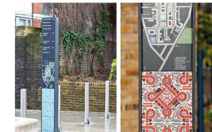
SI - SIGN - INFORMATION. SUPPLIER: IS GROUP. PRODUCT: WAY2GO TOTEM CONFIGURATION 3 OR 4. DIMENSIONS: H:2200MM X W:450 X D:140MM. AREA B - TOUGHENED GLASS OVER MAP. AREA D - POWDERCOATED WITH BLUE/TURQUOISE/GREEN. TO INCLUDE: • EACH BOARD WILL HAVE INFORMATION ON THAT PARTICULAR AREA. • OPEN TIME RESTRICTIONS IF ANY. • RULES FOR USING EACH SPACE. • CONTACT NUMBER TO REPORT ISSUES.
