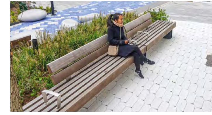
A LINEAR SEAT LOCATED WITHIN PLAY AREA. FSC CERTIFIED HARDWOOD. SUPPLIER: STREETLIFE OR EQUAL. PRODUCT: ROUGH AND READY 6 OR EQUAL WITH BACKREST & ARMRESTS. DIMENSIONS: L:2340MM SEAT HEIGHT: H:450MM. ROOT FIXED TO SUPPLIERS RECOMMENDATION.
