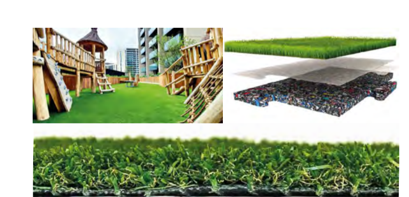
J SYNTHETIC GRASS. SUPPLIER: EASIGRASS, NAMGRASS OR EQUAL APPROVED. PRODUCT: HOLLAND PARK, ELISE OR EQUAL APPROVED. INSTALLED TO SUPPLIERS RECOMMENDATION WITH SHOCKPAD TO REQUIRED DEPTH TO ALLOW FOR PLAY EQUIPMENT FALL HEIGHTS. SUB-BASE TO ENGINEERS SPECIFICATION.
