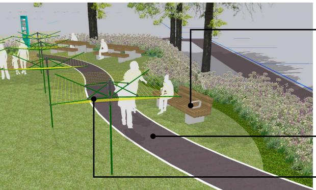
LINEAR SEAT LOCATED WITHIN PLAY AREA. FSC CERTIFIED HARDWOOD. SUPPLIER: STREETLIFE OR EQUAL. PRODUCT: ROUGH AND READY 6 OR EQUAL WITH BACKREST & ARMRESTS. DIMENSIONS: L:2340MM SEAT HEIGHT: H:450MM. ROOT FIXED TO SUPPLIERS RECOMMENDATION.
