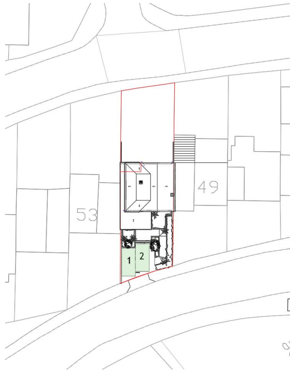
Fig 10. Two car parking spaces to be provided by the new driveway, with one space retained adjacent the rear dropped kerb. Creating three car parking spaces in total.
