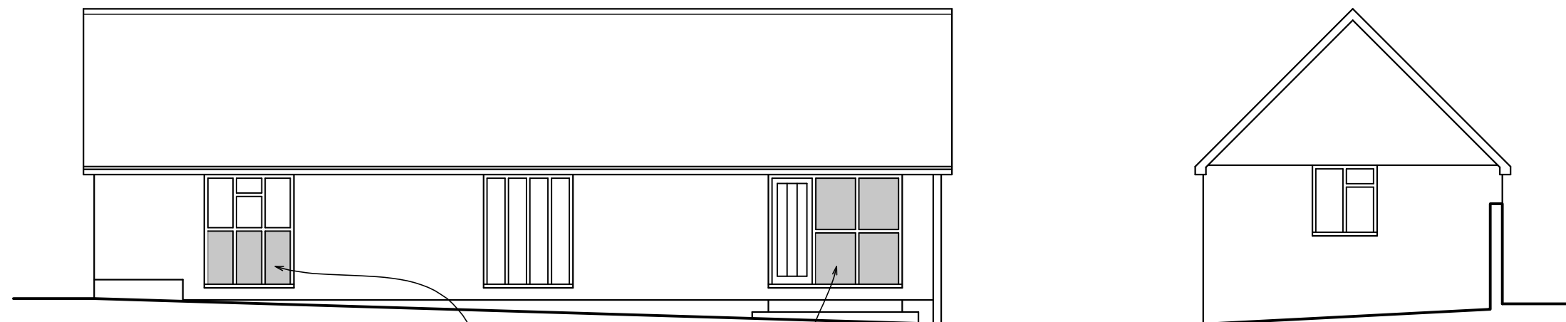
EAST ELEVATION AS PROPOSED SCALE: 1:100 NO CHANGE TO EXISTING WALL OR ROOF MATERIALS
