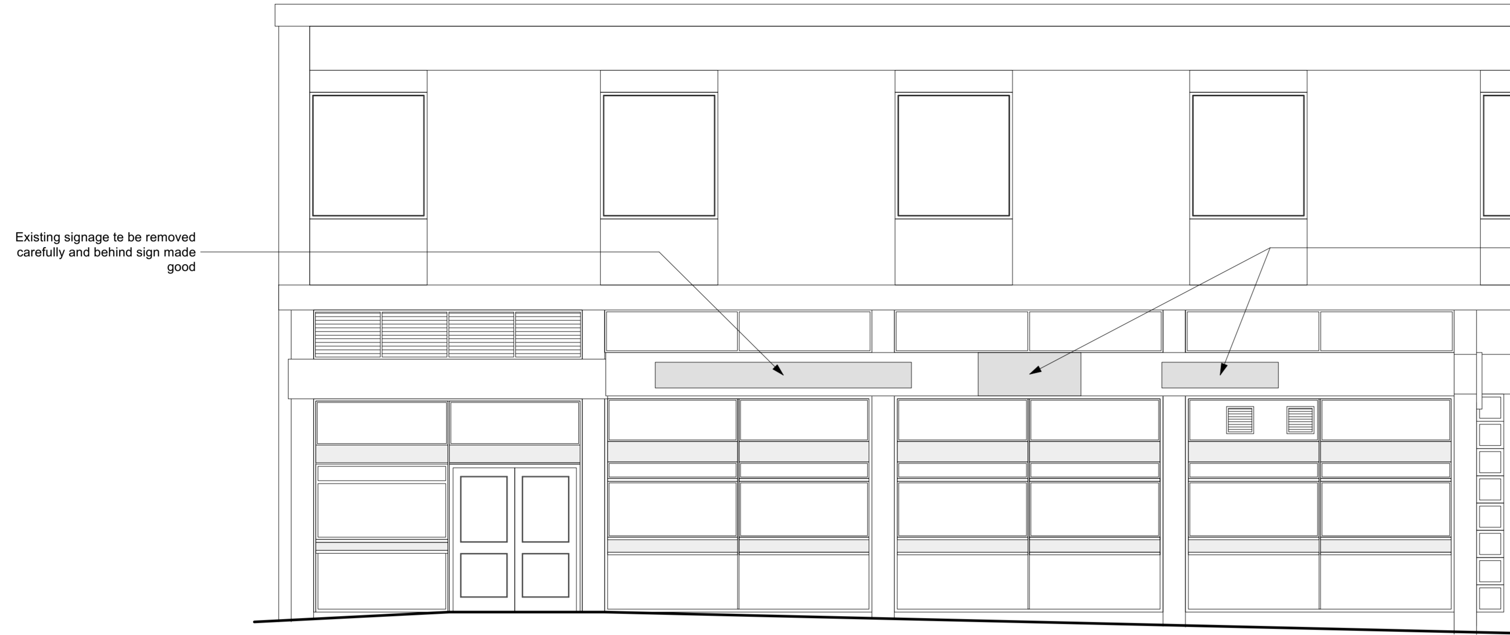
EXISTING ELEVATION Front Elevation
