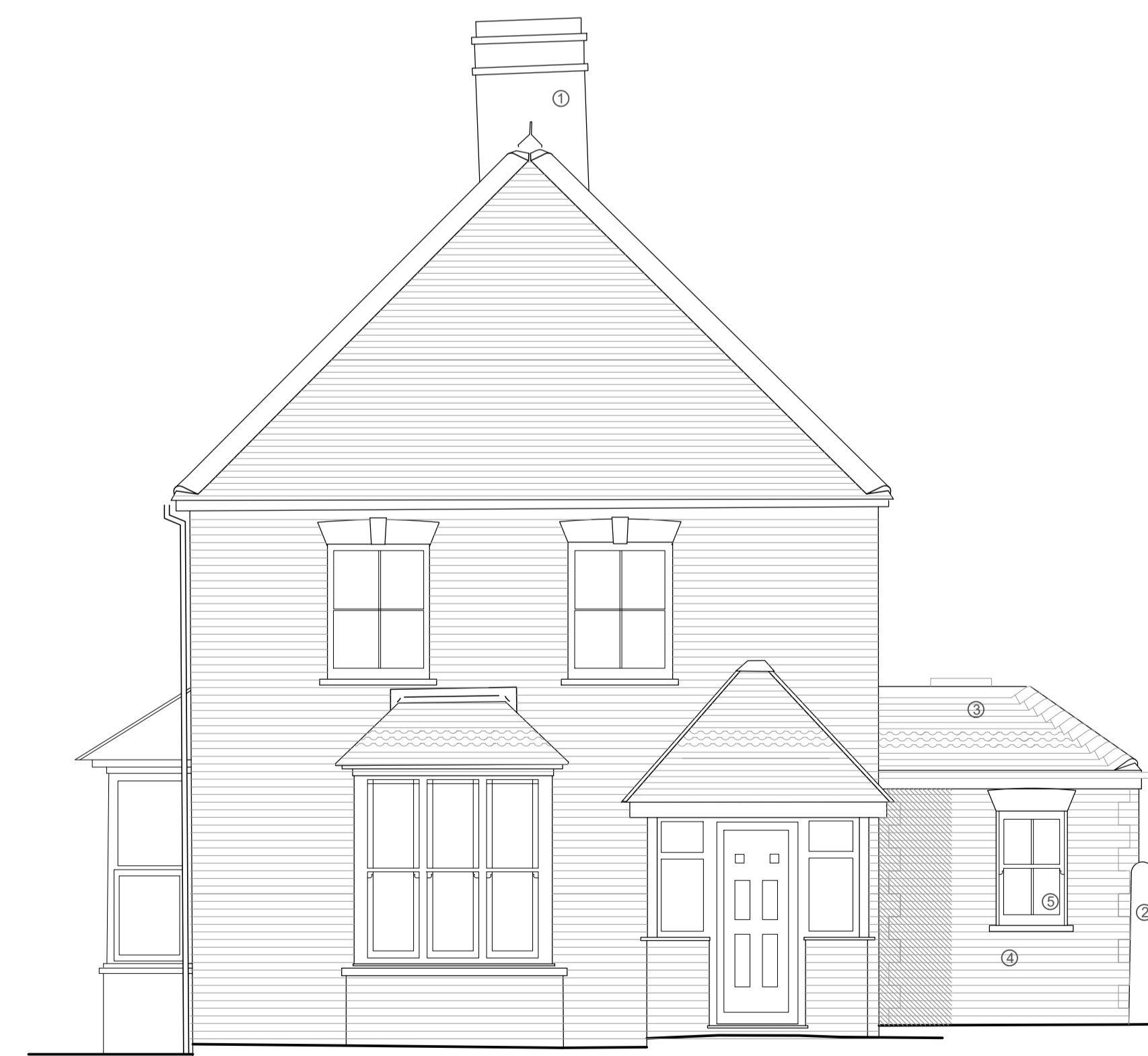
Proposed Eastern Elevation 1:50
