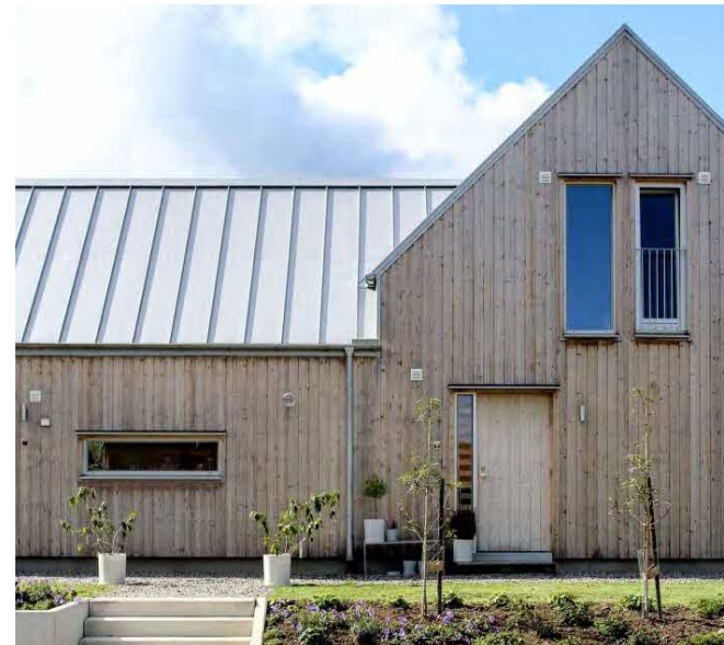
1. Light grey/natural metal standing seam roof
