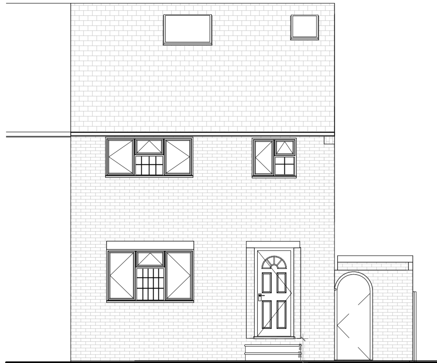
1 Existing Front Elevation 1 : 50
