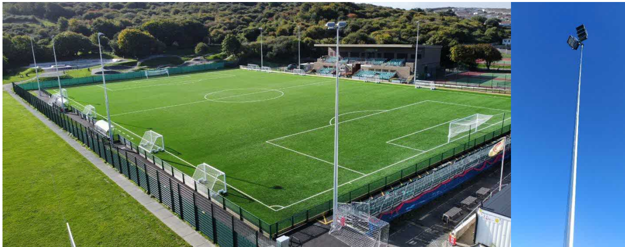
Figure 2 – Examples of 15m high slimline floodlighting column with LEDs (proposal is for 13m)
