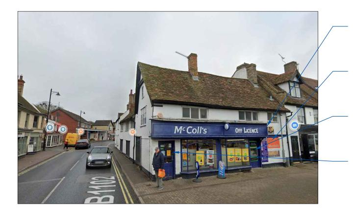
Remove existing plywood and sub frame, fit new sub frame to accommodate signage. New subframe, signage framing (inc soffits) to be painted. Colour: Grey
