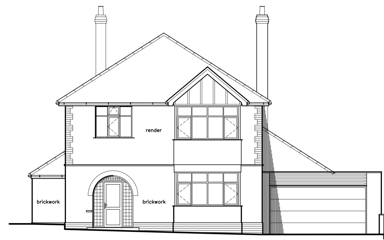
existing front elevation 1:100
