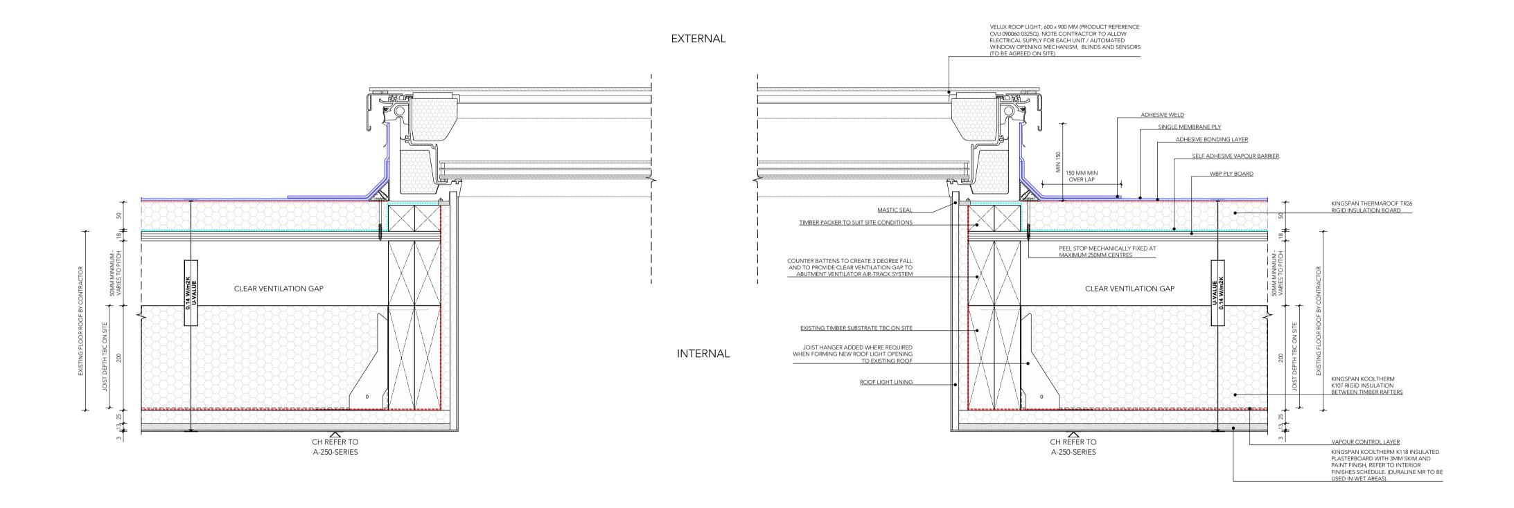
TYPICAL ROOFLIGHT DETAIL: SECTION
