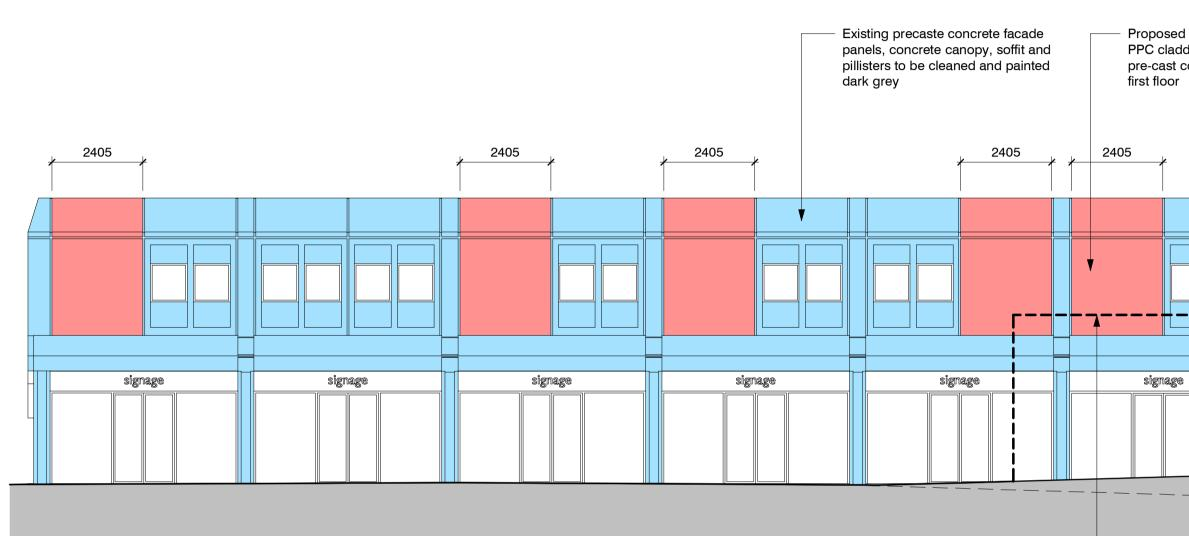
**10 First Floor Facade - Proposed South Elevation** 1:100
