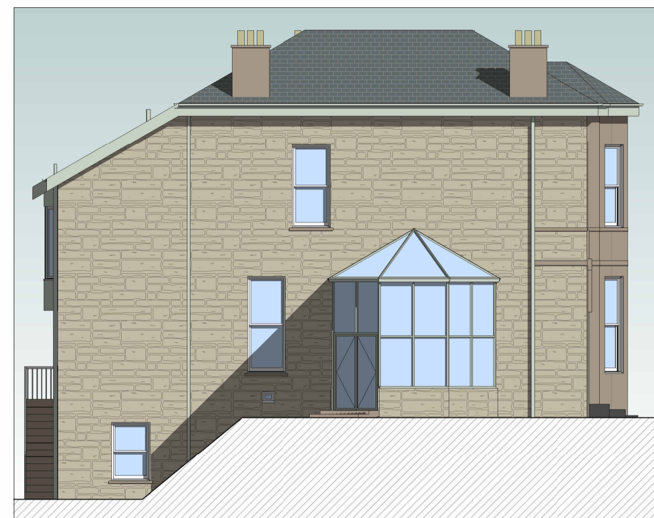
B ELEVATION B - AS EXISTING 1:100
