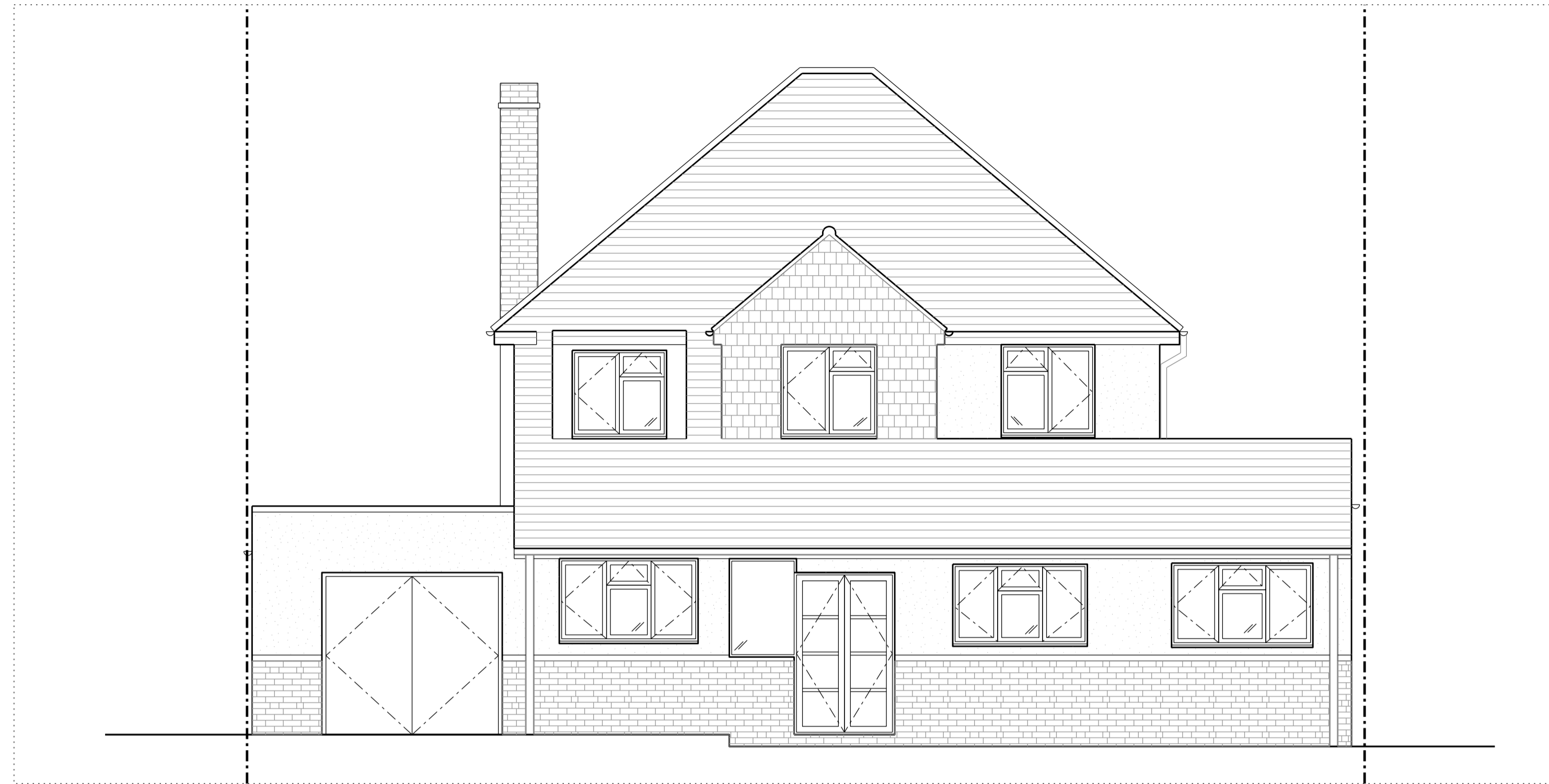
Existing Front Elevation
