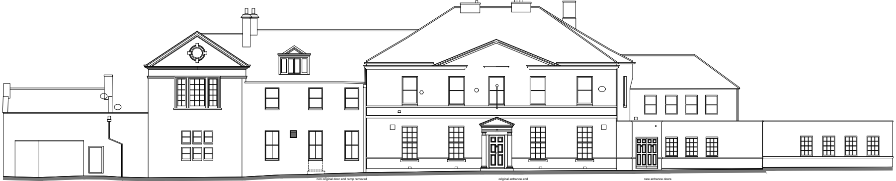
PROPOSED ELEVATION FACING SOUTH not original door and ramp removed new window to match existing, retained added new stonework lintel and sill to match existing frame profiles, panelling and details of window to match existing retained windows to either side original entrance and door to be retained door to be painted hardwood in a painted hardwood frame pannelled and lettered as shown with polished brass knocker and letter box new entrance doors to replace existing
