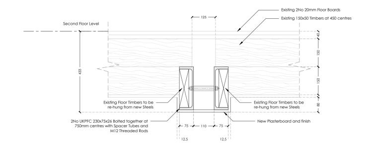
Existing Beam Arrangement (Elevation)
