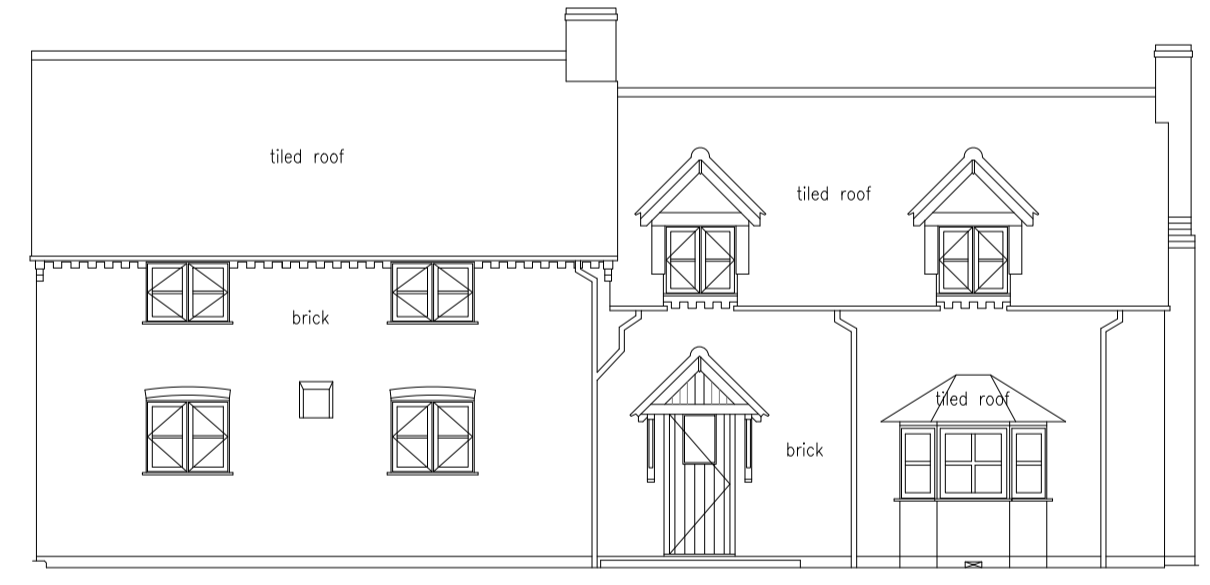
MAIN HOUSE EXISTING FRONT ELEVATION Scale 1:100
