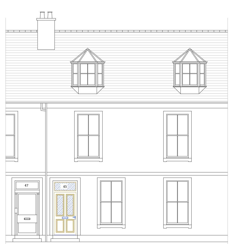
New hardwood door and frames, to be fitted to existing opening in granite wall. Door and glazing beads etc. to be painted dark blue, with hardwood frames painted white. Internal surface of door and frames etc. to be painted white.
