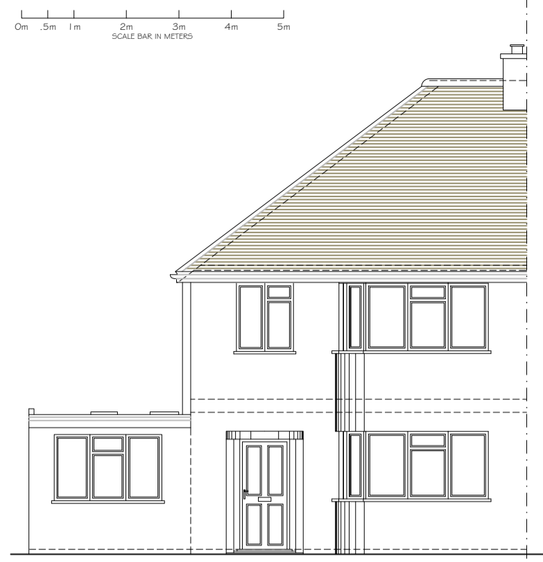
EXISTING FRONT ELEVATION
