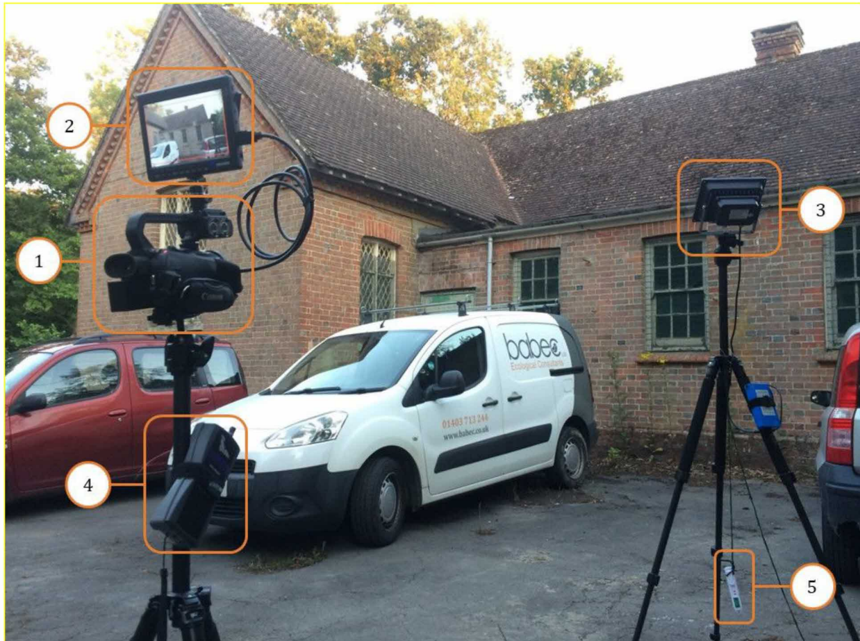
1. Canon XA series camcorder 2. Screen 3. Infrared floodlamp 4. Batlogger-M 5. Thermometer
