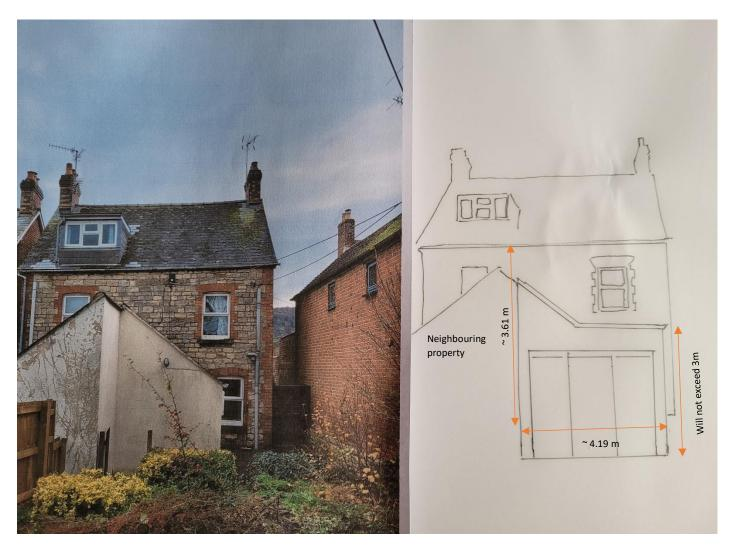
Whilst the exact design of the extension is yet to be finalised, the height of the proposed extension will not exceed a height of 3m.
