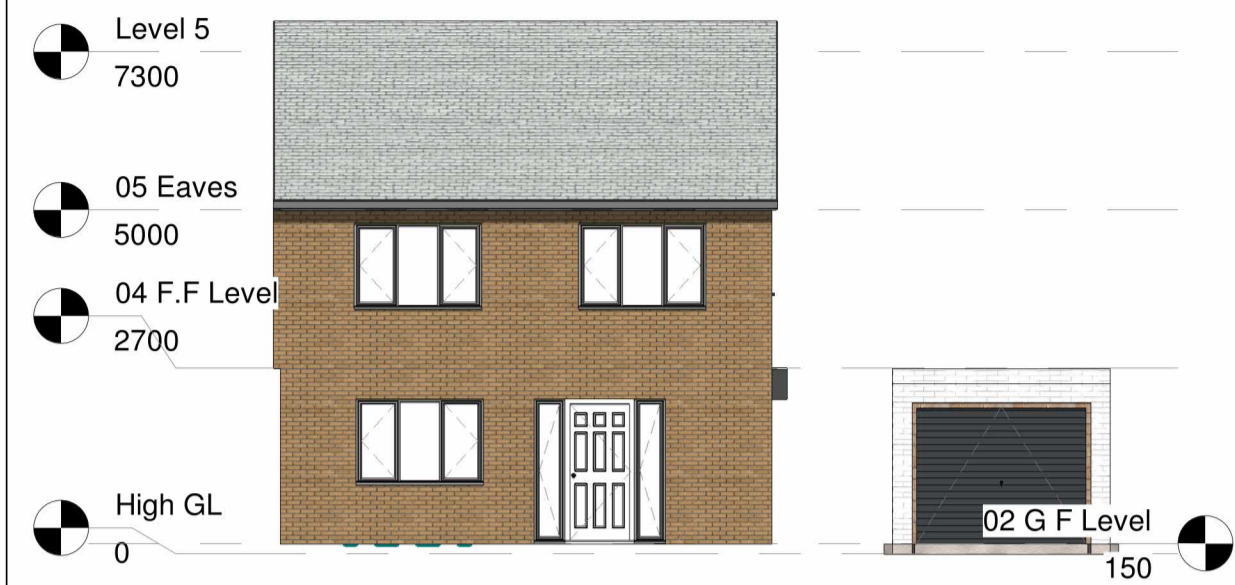
Existing North Elevation 1 : 100
