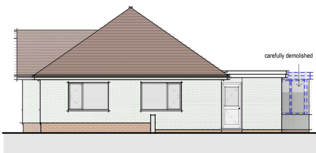
4 existing south elevation 1 : 100
