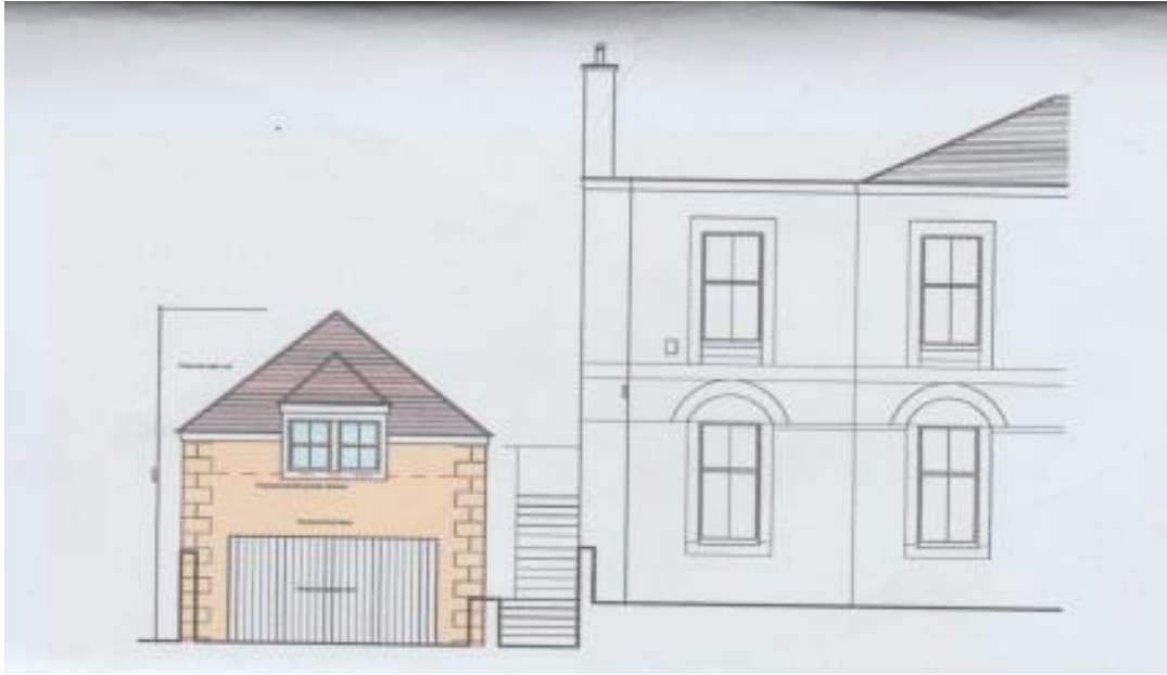
Elevation of previous planning consented building Frontage 6.2m Height 6.35m GIA 87.6SQM
