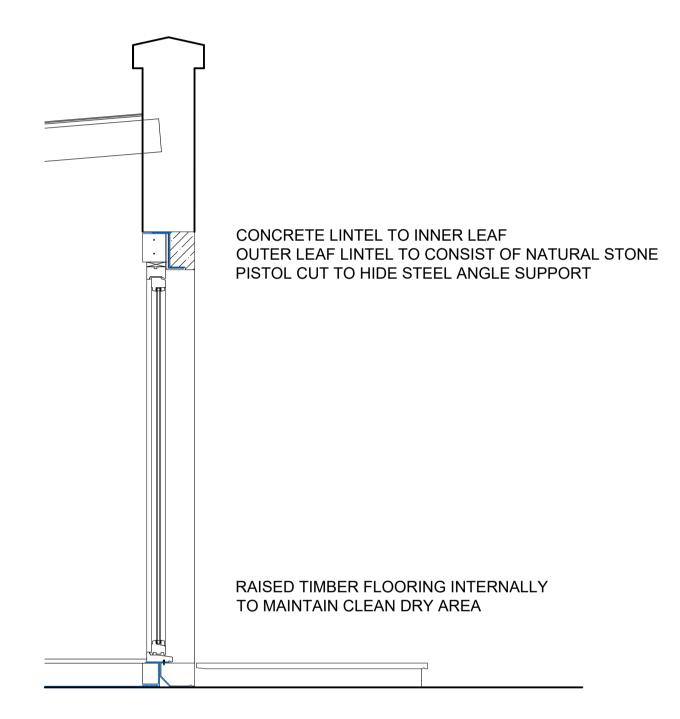
EXTERNAL PLATFORM TO CONSIST OF 40mm THICK NATURAL SLATE PAVING SLABS ON CONCRETE SCREED/ STONE CHIP SURROUND
