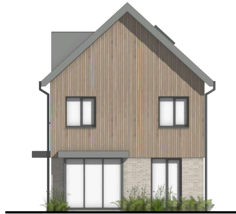
House 1 - North Elevation Scale 1: 100
