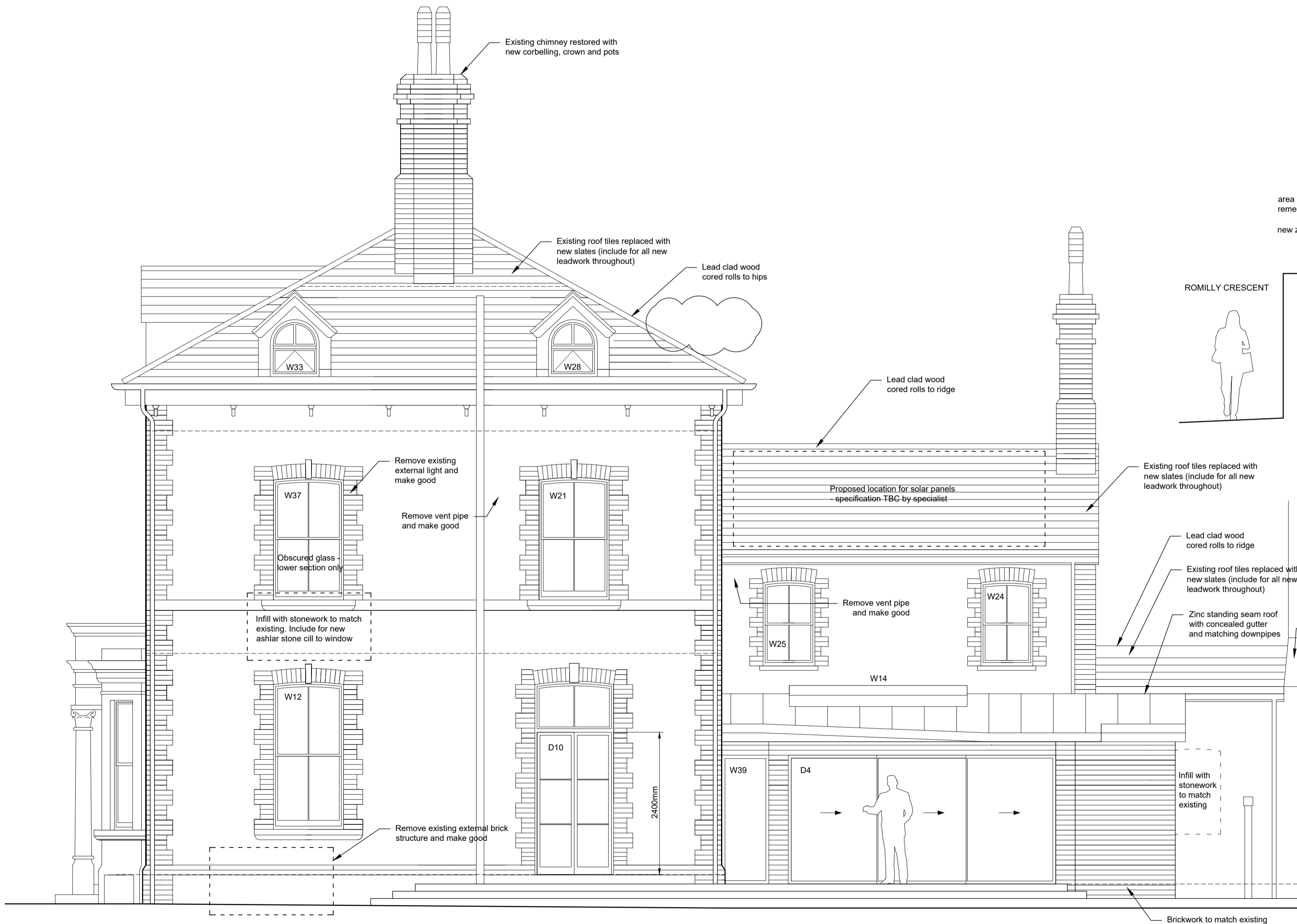
SOUTH ELEVATION at 1:50
