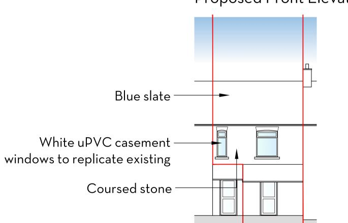
Poor condition timber windows to be replaced with white timber effect uPVC to replicate style and size of existing.
