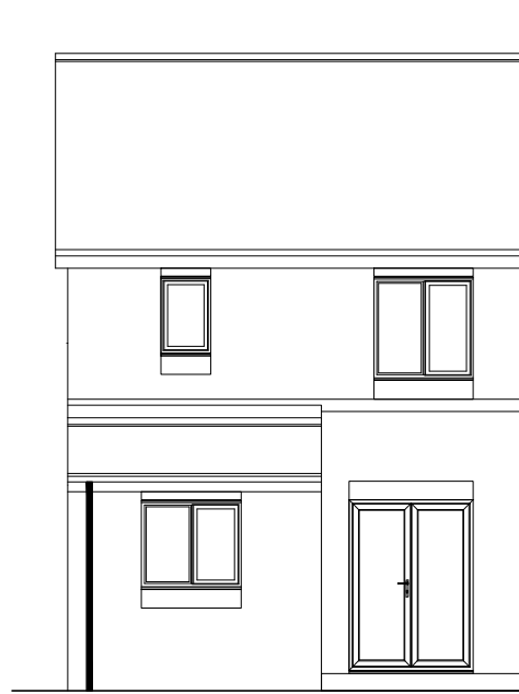
EXISTING REAR ELEVATION
