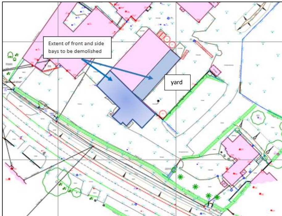
Figure 3 – Bays Proposed for demolition
