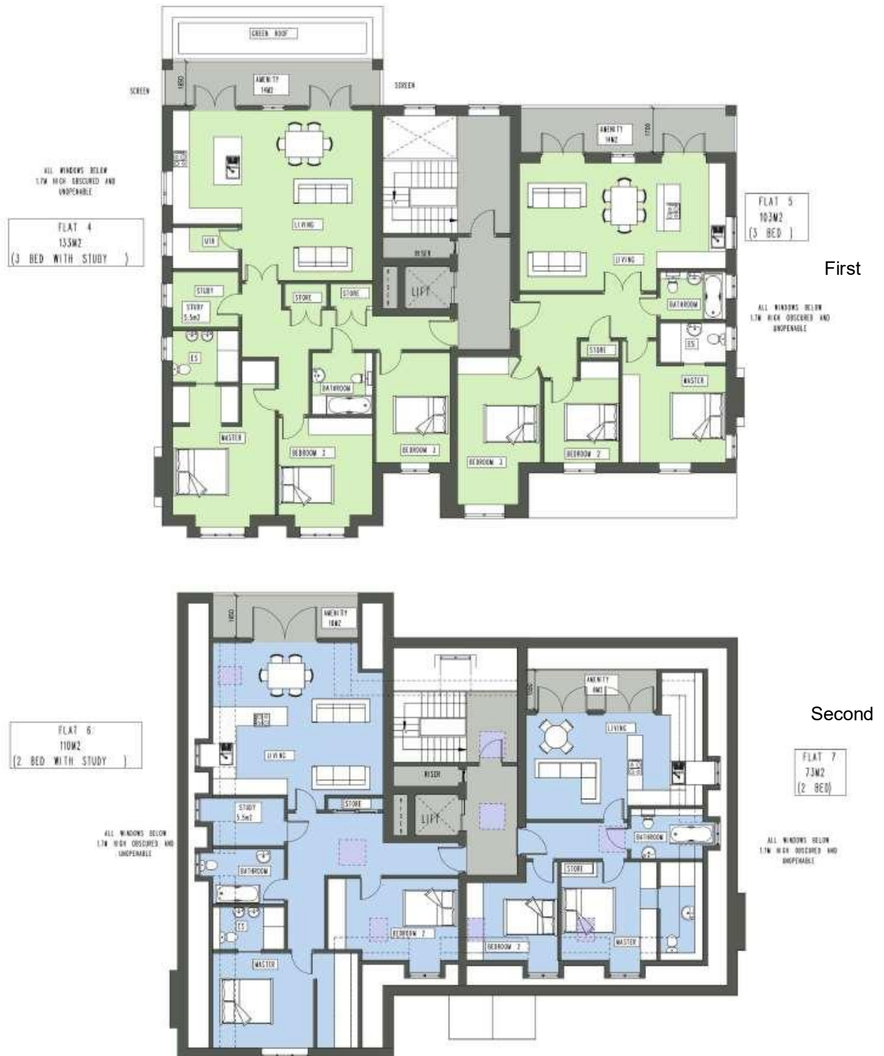
Figure 6: Layouts of the lower ground to second floors of the proposed development. Habitable rooms are analysed for daylight provision and sunlight.
