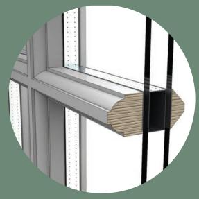
Simulated divided lights to visually match original glazing bars. No thermal breaks around the perimeter of the glazing bars. Discreet double glazing with white back to back spacer bars, period mouldings and outer beads to match angled putty lines.
