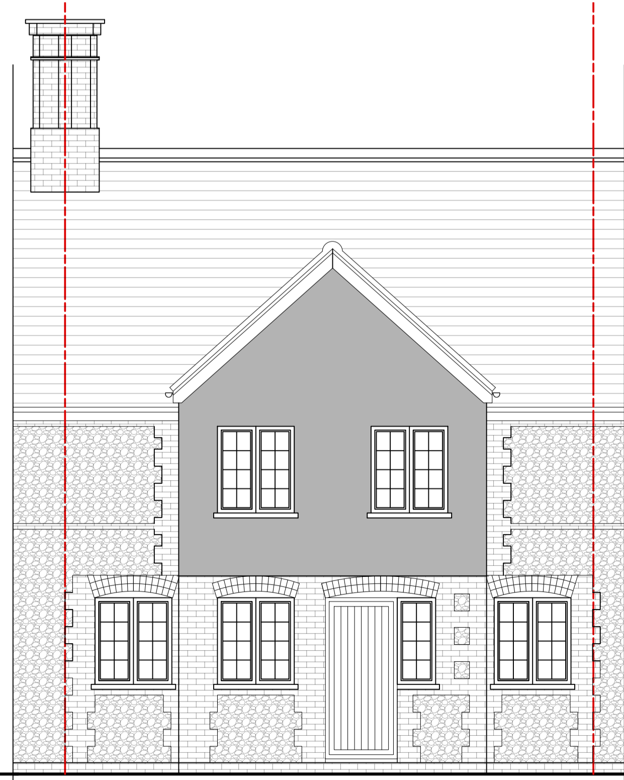
EXISTING SOUTH ELEVATION 1:50
