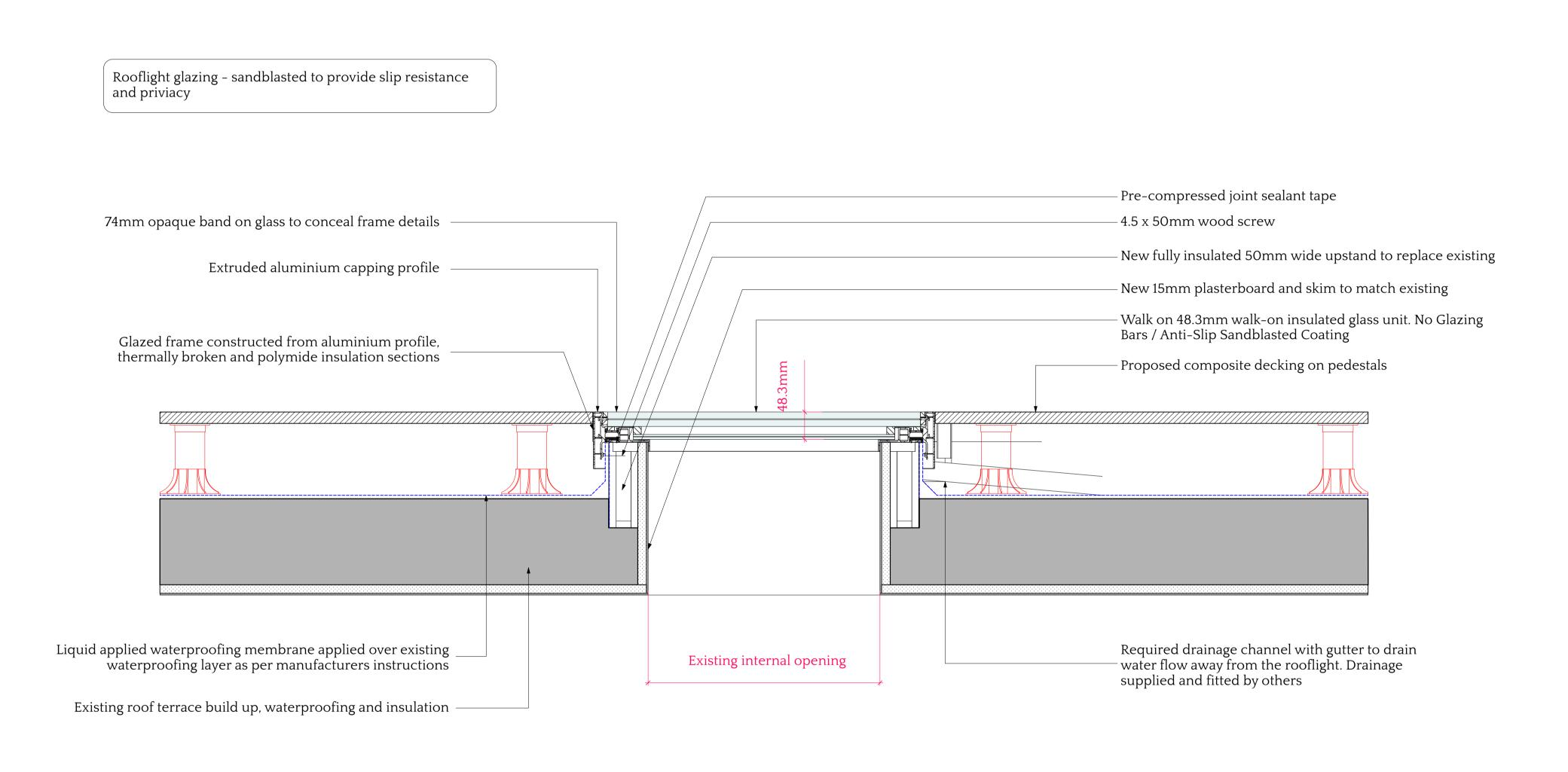
1 Proposed Rooflight Detail - NRL.01.02 Scale: 1:5
