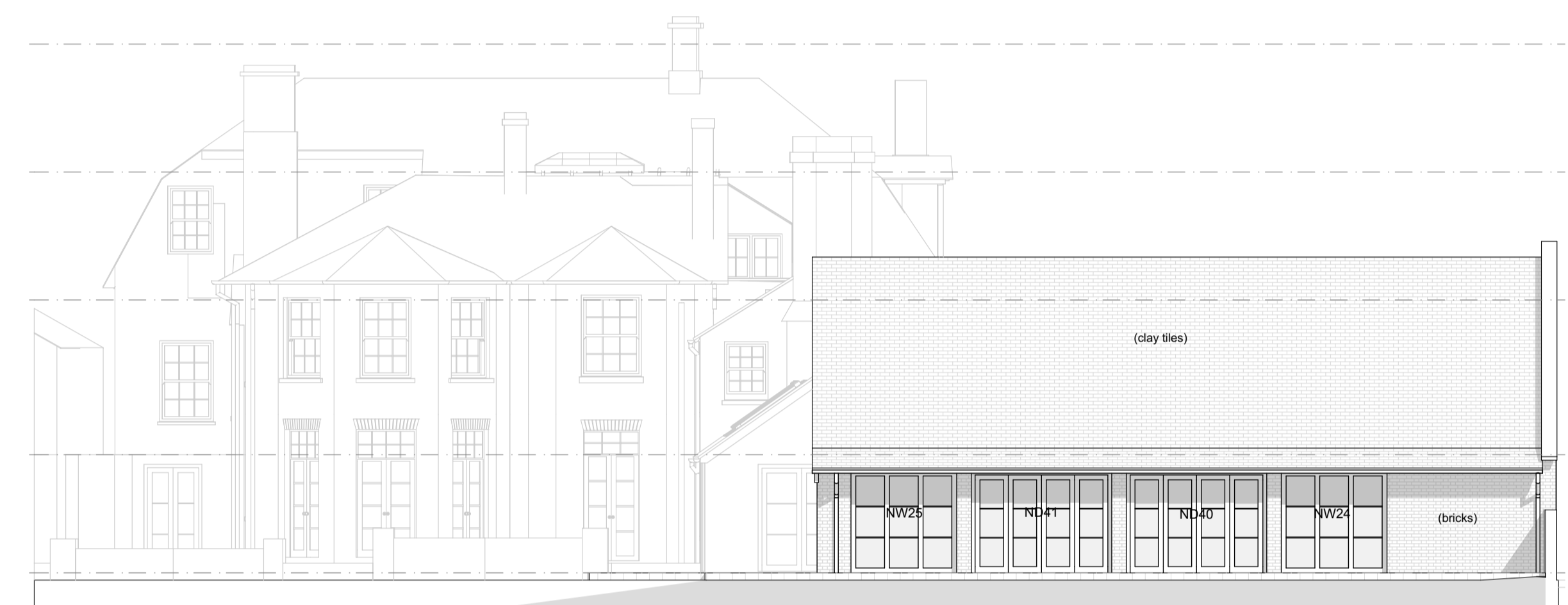
Swimming Pool - North Elevation - Proposed 1:100
