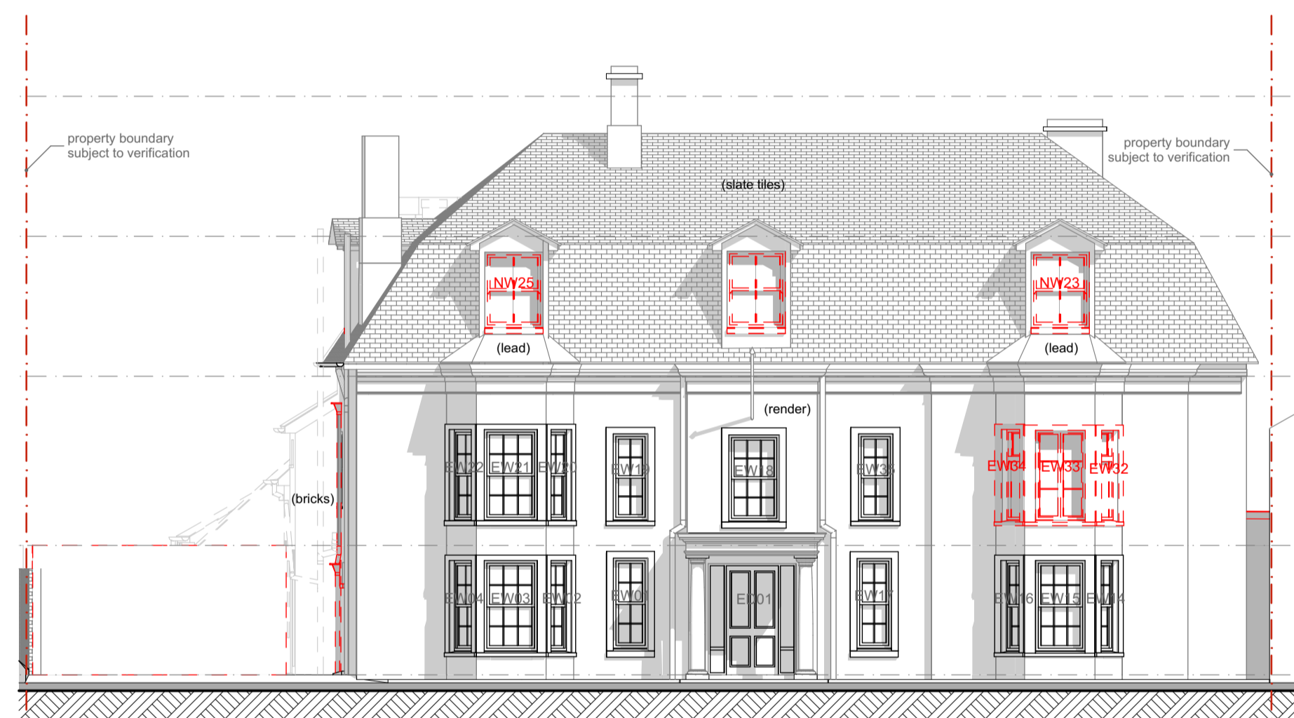
South Elevation - Removals 1:100
