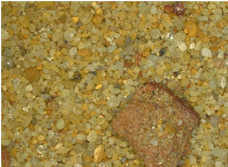
5678 insolubles >45µm Stereomicroscope x10
