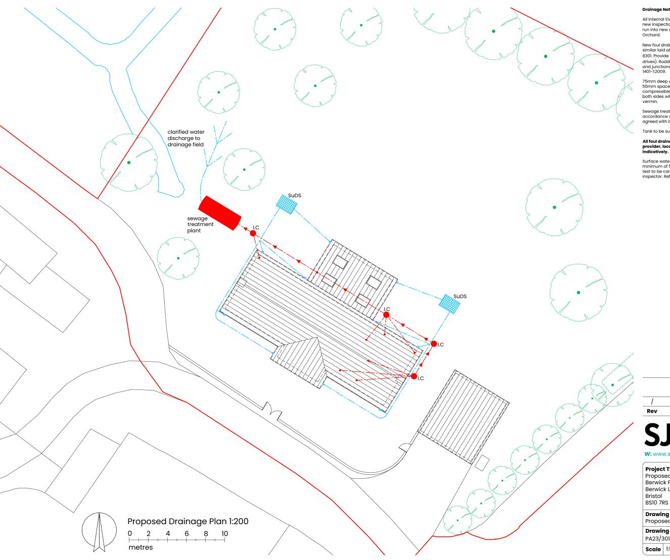
All Internal SVPs and floor sockets for foul waste to connect into new inspection chambers as shown. New Inspection chambers to run into new sewage treatment plant / septic tank located in Orchard.
