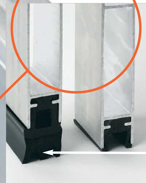
Flood Boards MG_4401/4 Cross section of boards. Each flood board is 400mm high x 25mm thick and is supplied with rubber seals to prevent water ingress.
