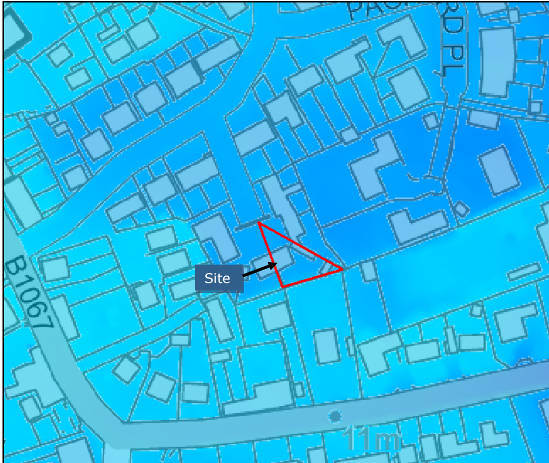
Figure 2: Filtered LIDAR survey data at 1m resolution where higher ground is denoted by red and orange colours and lower ground is denoted by blue colours
