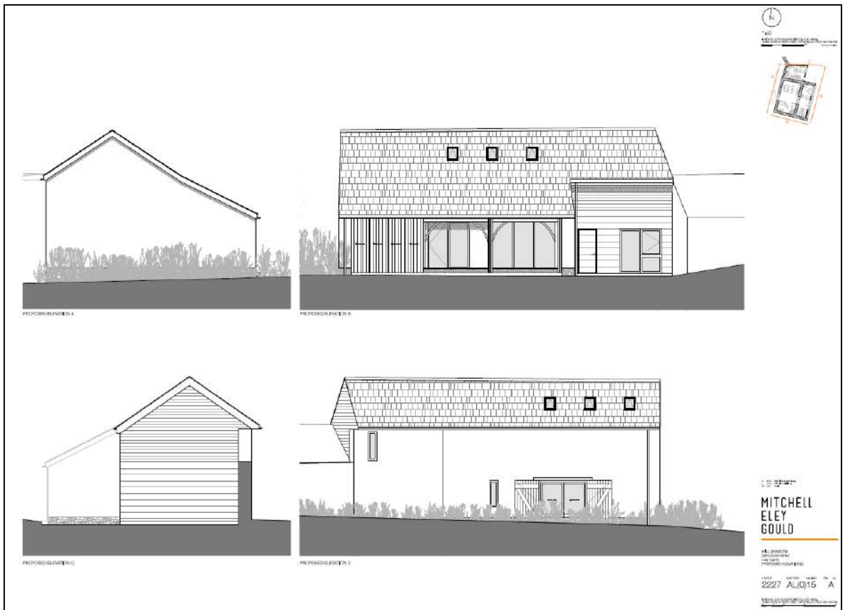
Figure 2-5: Proposed elevations of the hay barn, Barn 1
