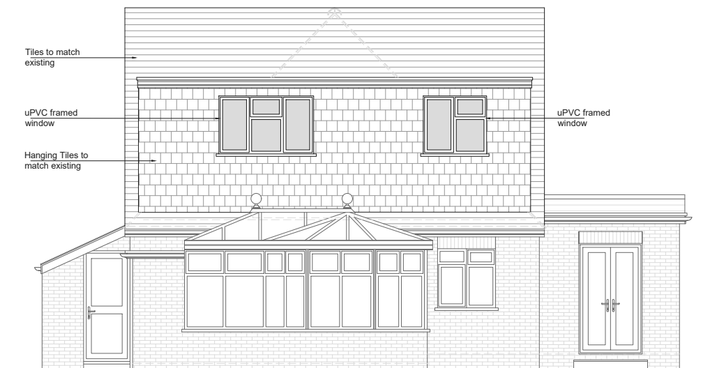
PROPOSED REAR ELEVATION SCALE 1:100
