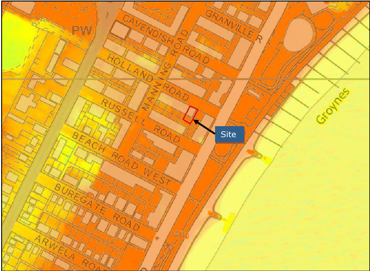
Figure 2: LIDAR survey data where higher ground is denoted as red, orange and yellow colours and lower areas denoted by blue and green colours
