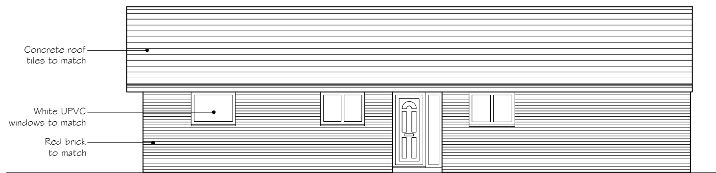
Proposed Side (North West) Elevation (1:100)
